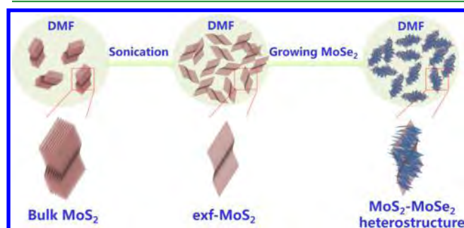
Figure 1. Schematic illustration of the synthesis route for vertically aligned MoS 2 –MoSe 2 heterostructures.
